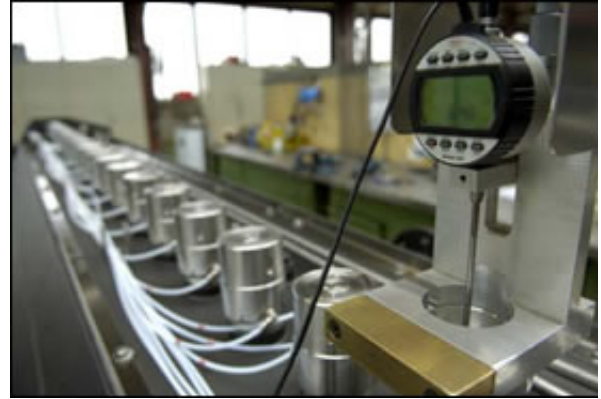
Calibration of every zone control valve.
