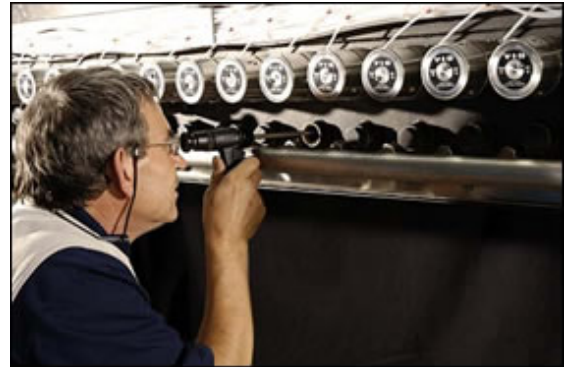
Thorough inspection through maintenance and cleaning openings.
