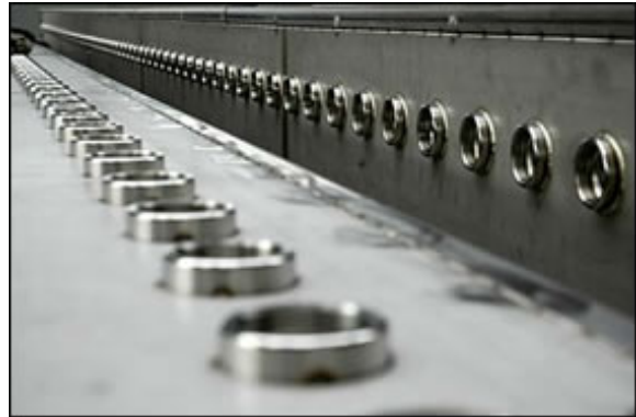
Two different VIB SmoothTech profilers before further treatment in the pickling plant.
