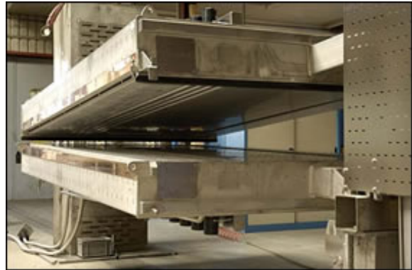
The one-sided pneumatic retraction unit opens, when required, both units of the VIB MoistureTech.
