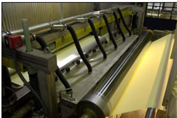
A complete MoistureTech system from VIB Systems – here two-sided moistening of thermal paper at a production speed of 1,300 m/min (4,250 fpm).
